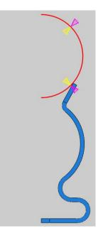
As a surface can contact on either side, so it is important to specify the desired side of the surface to be in contact. It is done by choosing the color associated with the desired side.
