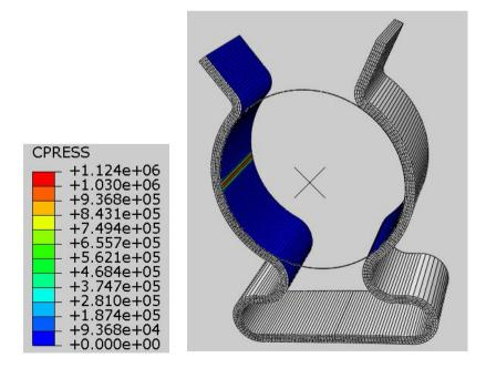
It can be seen that contact pressure develops only in a small region between the fuse and the holder.
