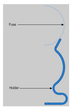
The model consists of two two-dimensional parts: fuse and holder. The fuse is modeled as an analytical rigid part. The holder is assumed to be made from brass with a Young's modulus of 100 GPa and a Poisson's ratio of 0.3. It is assumed that contact is frictionless. The holder is meshed with bilinear plane strain quadrilateral elements with reduced integration (CPE4R).
