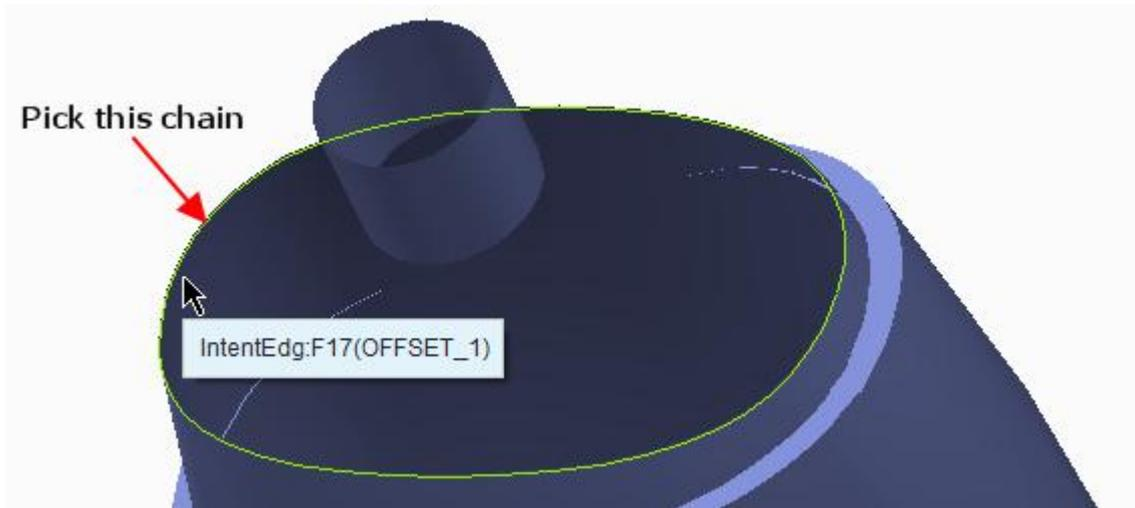
Now hold down the Ctrl key and pick the second chain using the Intent chain technique as shown below.
