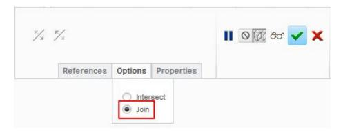
Join option is used when two surfaces have a common edge. Join option is faster than Intersect option.
