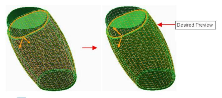
Pick or middle-click after making sure that arrows direction is as shown in the above figure. Now the part should appear as shown below. (If not then go back and fix it)
