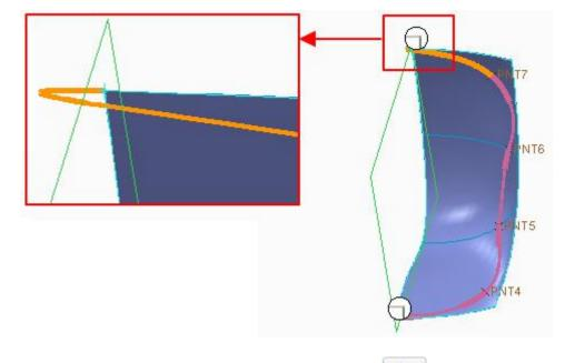
It is due to the wrong direction of normal constraint. So pick **Flip** to reverse the direction.
