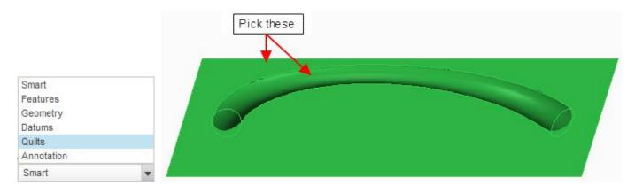
Pick <sup>O Merge</sup> on the Model tab to invoke Merge tool.
