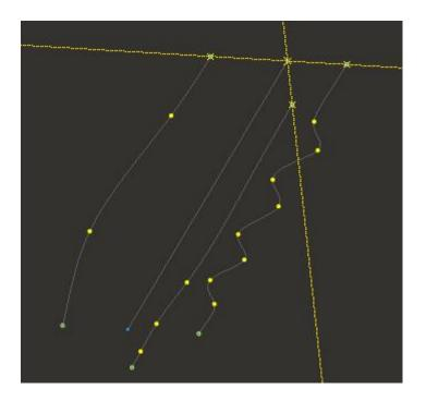
Pick  $\sim$  spline and sketch a three point spline that passes through the references for chains as shown below (View shown after picking ).
