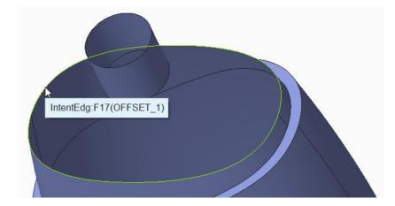
Now hold down the Ctrl key and pick the second chain using the Intent chain technique as shown below.
