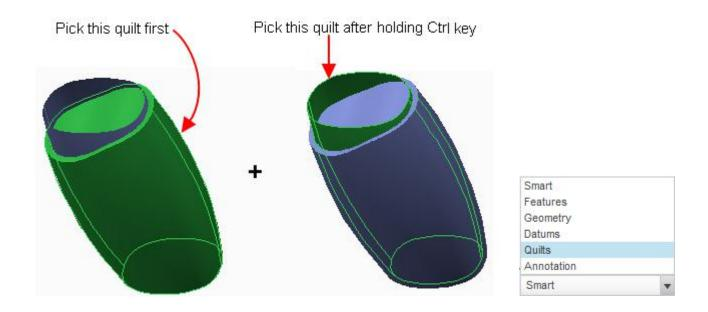
Pick <sup>Merge</sup> to invoke Merge tool and then <sup>X</sup> so that preview appears as shown below. (Notice the direction of arrows)
