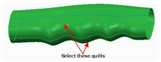
Pick <sup>Merge</sup> on the Model tab to invoke Merge tool.
