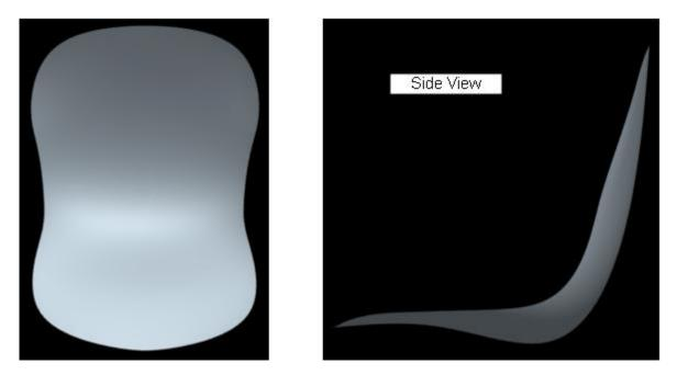
Set the working directory to the EXAMPLES folder and open the model CHAIR.PRT. Because this part is symmetrical so we will create half side of the part and then mirror it. Required datum curves have already been created. You are encouraged to explore the way these curves have been defined after completing this exercise.
