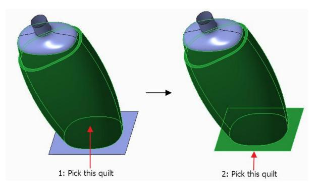
Pick <sup>Merge</sup> on the Model tab to invoke Merge tool and preview will appear as shown below.
