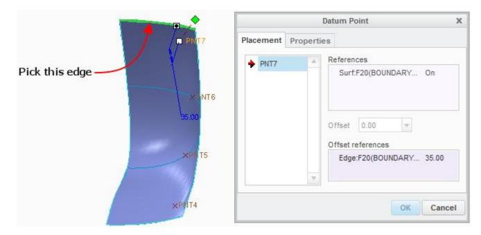
Hold down the Ctrl key and select the side edge as second offset reference. Enter **35** as the Offset value as shown below.
