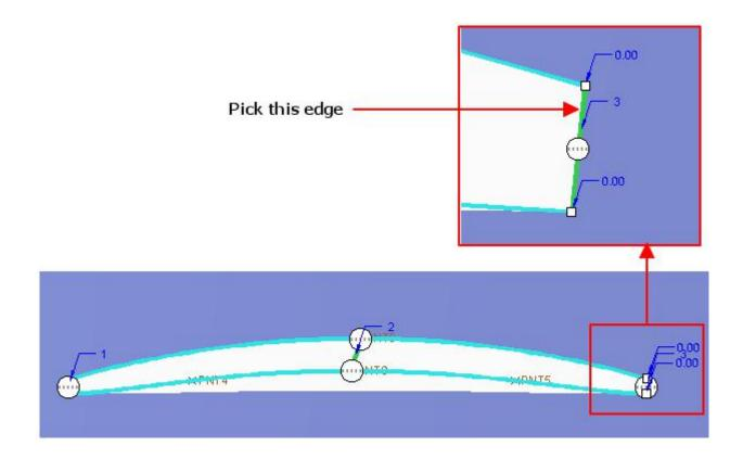
Apply the **Tangent** constraints for the three chains as shown below.
