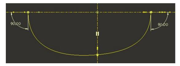
To add spline tangency dimension at a point, click the spline, then click the geometry to which the spline tangency is to be defined and then click the endpoint where the tangency is to be defined. Then click the middle mouse button to place the dimension.
