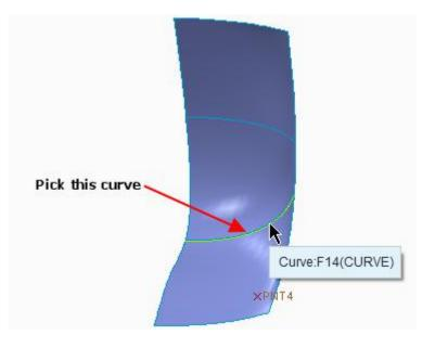
Pick Next End to change the measurement reference to right end of curve
