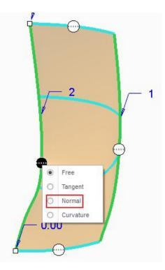
This surface will be mirrored about RIGHT datum plane. Therefore to maintain tangency between original and mirrored surface, the surface has been constrained Normal to the RIGHT datum plane.
