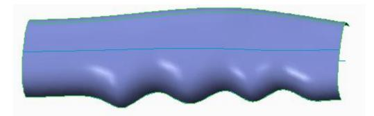
Notice that cross-section remains aligned to the chains all along the sweep feature.
