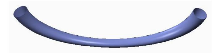
Now we need to close the open ends so that quilt can be converted to a solid. For this, we will merge an extruded surface with the swept surface. The extruded surface has already been created but hidden.
