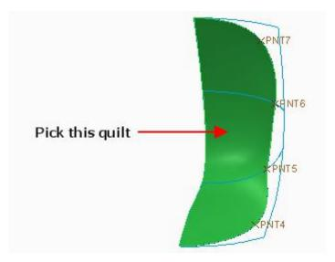
Pick Mirror on the Model tab to invoke Mirror tool and select the **RIGHT** datum as Mirror plane.
