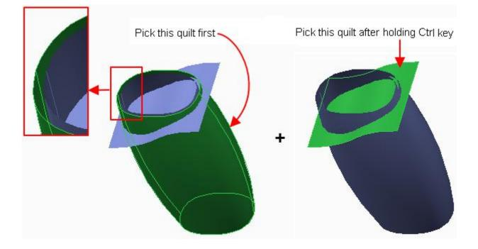
Pick <sup>Merge</sup> on the Model tab to invoke Merge tool and preview will appear as shown below.
