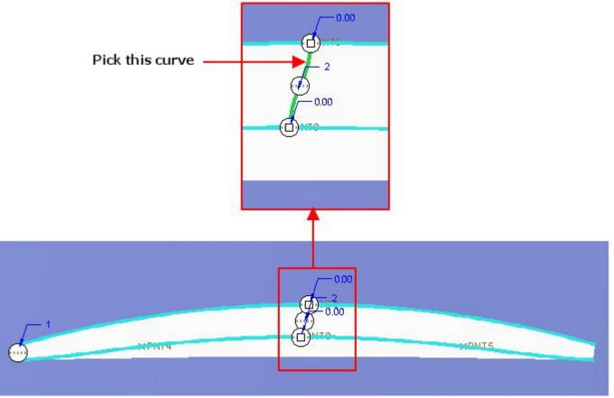
While holding down the Ctrl key, pick the edge, shown in the figure below as last chain in second direction.
