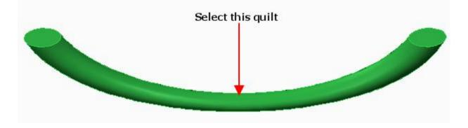
Pick Solidify on the Model tab to invoke Solidify tool.
