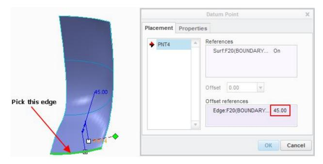
Hold down the Ctrl key and select the side edge as second offset reference. Enter **25** as the Offset value as shown below.
