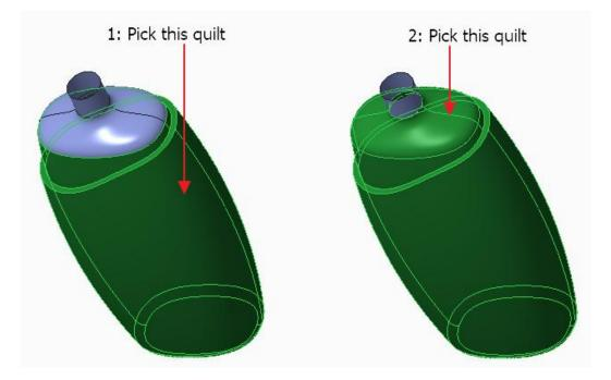
Pick <sup>Merge</sup> on the Model tab to invoke Merge tool.
