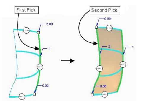
Apply the **Normal** constraint for the chain that lies on RIGHT datum plane as shown below.
