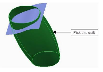
Pick Offset on the Model tab to invoke Offset tool and enter **2** as the offset value on the dashboard.
