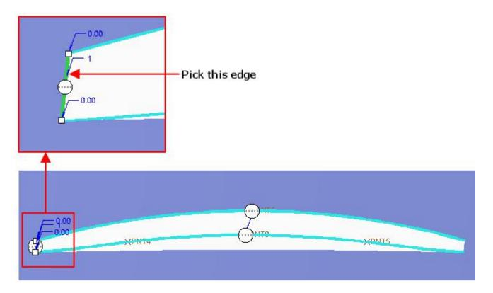
Now hold down the Ctrl key and pick the datum curve, shown in the figure below as second chain in second direction.
