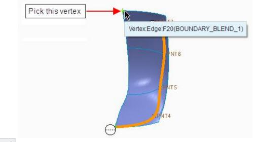
Pick Placement to access the Placement panel and check the 'Place curve on surface' option.
