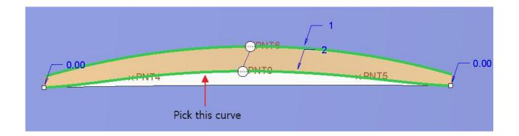
Pick in the 'Second direction' collector to activate either on dashboard or in Curves panel.
