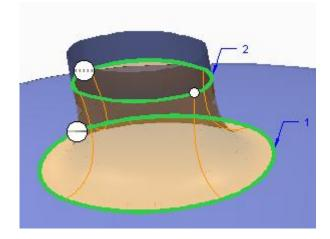
Apply the **Tangent** constraint for second chains as shown below.
