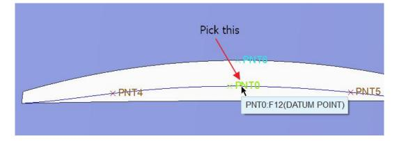
Now we will specify the tangent constraints for the ends of the curve.
