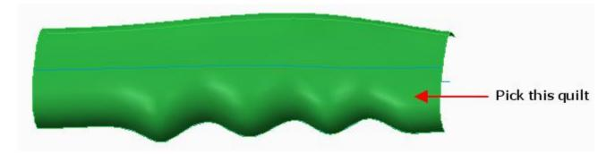
While the surface geometry is selected, pick Mirror on the Model tab to invoke the Mirror tool. Select the **FRONT** datum as Mirror plane.
