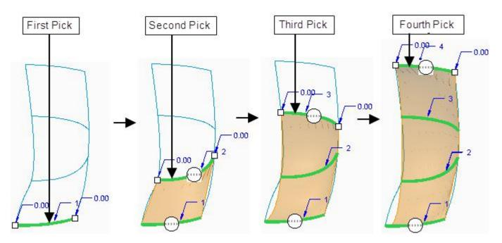
Pick in the Second Direction Collector to activate it and while holding down the Ctrl key, select the curves shown in figure below.
