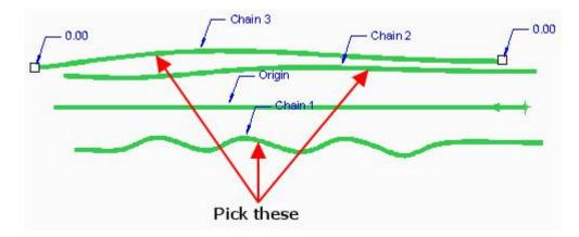
The order, in which chains are selected have no effect on the sweep geometry. Only the desired Origin Trajectory should be selected first.
