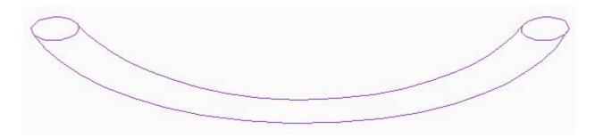
Notice that the joint between both quilts appears magenta which means that both surfaces have been merged into a single quilt.
