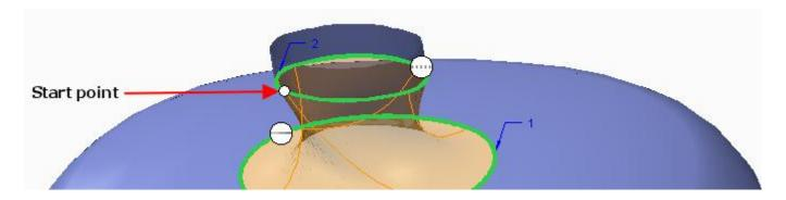
If you compare the location of Start Point for first and second chain then you can easily conclude that surface is distorted due to mismatch of Start Points. So we will change the location of Start Point of second chain so that it corresponds to the Start Point of first Chain.
