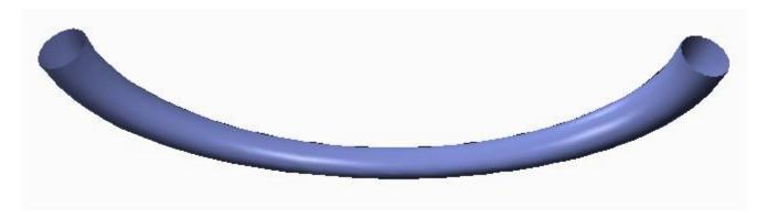
Now we need to close the open ends so that quilt can be converted to a solid. For this, we will merge an extruded surface with the swept surface. The extruded surface has already been created but hidden.
