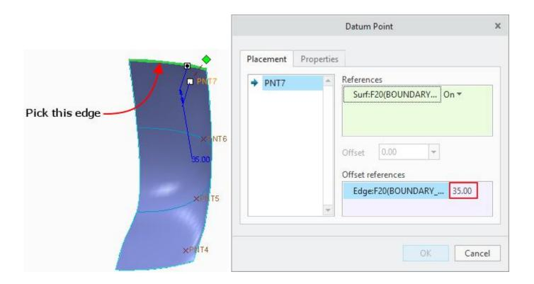
Hold down the Ctrl key and select the side edge as second offset reference. Enter **35** as the Offset value as shown below.
