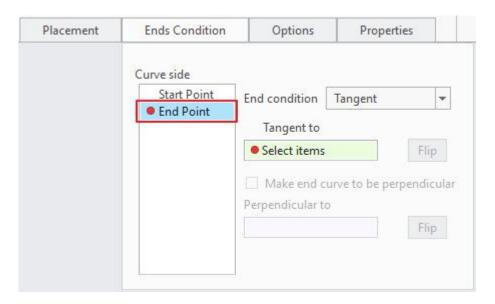
Again pick the following surface to make the new datum curve tangent to it at the end point.
