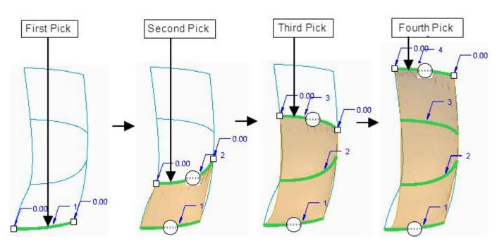
Pick in the Second Direction Collector to activate it and while holding down the Ctrl key, select the curves shown in figure below.
