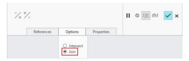
Join option is used when two surfaces have a common edge. Join option is faster than Intersect option.
