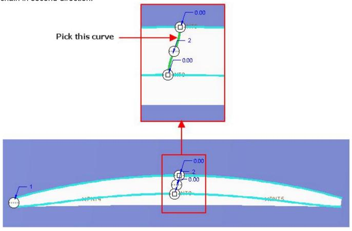
While holding down the Ctrl key, pick the edge, shown in the figure below as last chain in second direction.
