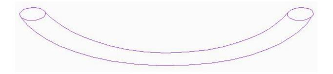
Notice that the joint between both quilts appears magenta which means that both surfaces have been merged into a single quilt.
