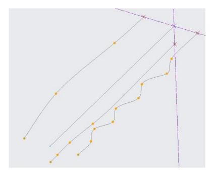
Pick Spline and sketch a three point spline that passes through the references for chains as shown below (View shown after picking ).
