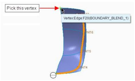
Pick Placement to access the Placement panel and check the 'Place curve on surface' option.
