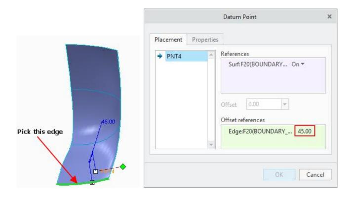
Hold down the Ctrl key and select the side edge as second offset reference. Enter **25** as the Offset value as shown below.
