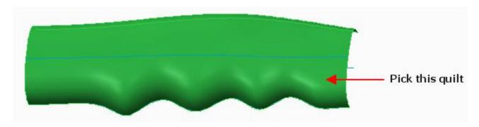
While the surface geometry is selected, pick Mirror on the Model tab to invoke the Mirror tool.
