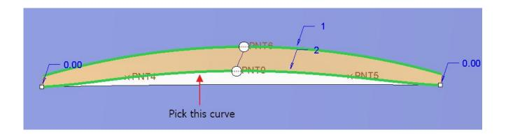
Pick in the 'Second direction' collector to activate either on dashboard or in Curves panel.
