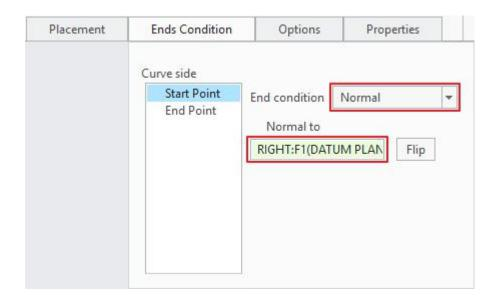
Change end condition for 'End Point' to Normal and select the RIGHT datum plane as reference.
