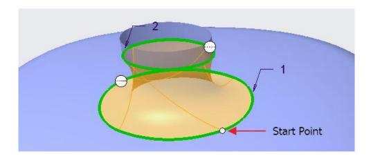
Pick Curves tab to view Curves slide-up panel. Here pick on the second chain as shown below.
