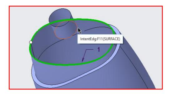
If the preview of surface appears distorted, then fix it before proceeding. The procedure to fix the distorted boundary blended surface was explained in previous exercise.
