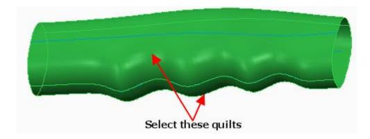
Pick Merge on the Model tab to invoke Merge tool.
