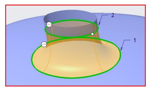
Apply the **Tangent** constraint for second chains as shown below.
