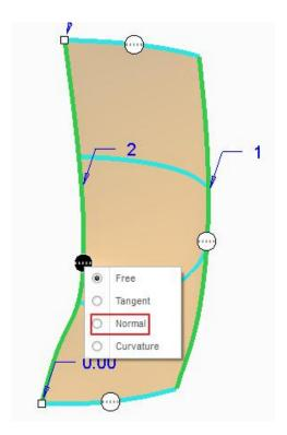
This surface will be mirrored about RIGHT datum plane. Therefore to maintain tangency between original and mirrored surface, the surface has been constrained Normal to the RIGHT datum plane.
