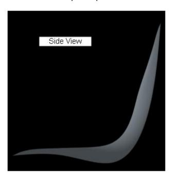
Set the working directory to the EXAMPLES folder and open the model CHAIR.PRT. Because this part is symmetrical so we will create half side of the part and then mirror it. Required datum curves have already been created. You are encouraged to explore the way these curves have been defined after completing this exercise.
