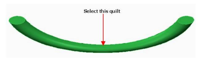
Pick Solidify on the Model tab to invoke Solidify tool.
