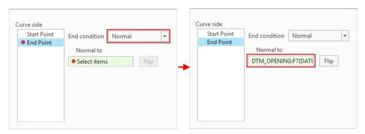
Select Flip to reverse the direction so that curve appears as shown in figure below.
