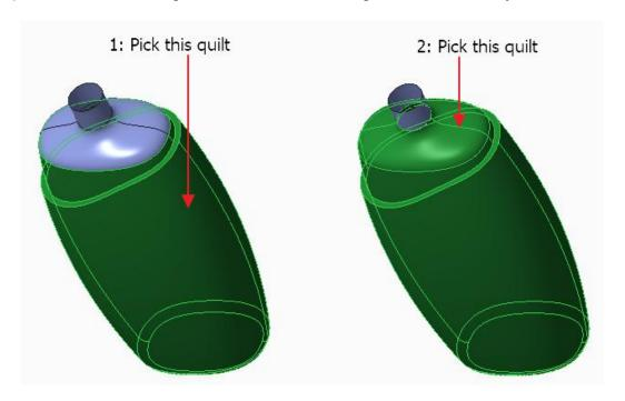
Pick Merge on the Model tab to invoke Merge tool.
