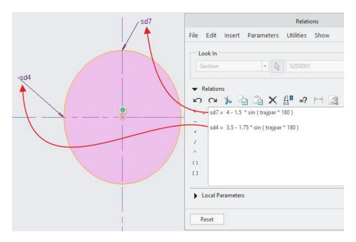
Using the trajectory parameter, trajpar, in a relation for a sweep feature allows to map any function, along the Origin Trajectory. The value of trajpar changes from 0 to 1 as the section is swept along the Origin Trajectory from start to end.
