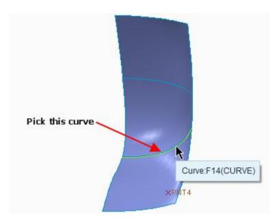
Pick Next End to change the measurement reference to right end of curve
