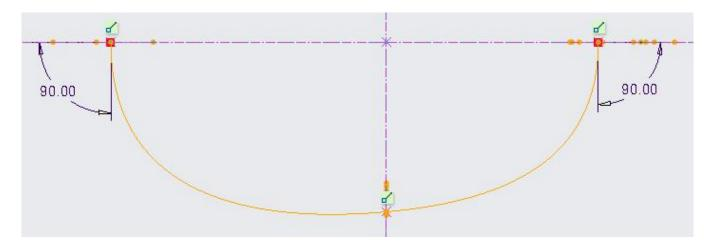
To add spline tangency dimension at a point, click the spline, then click the geometry to which the spline tangency is to be defined and then click the endpoint where the tangency is to be defined. Then click the middle mouse button to place the dimension.
