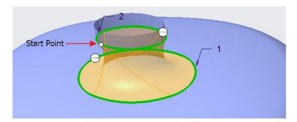
If you compare the location of Start Point for first and second chain then you can easily conclude that surface is distorted due to mismatch of Start Points. So we will change the location of Start Point of second chain so that it corresponds to the Start Point of first Chain.
