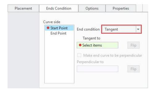
Now system wants to know a reference to which the new curve will be tangent, so pick the following surface to make the new datum curve tangent to it.
