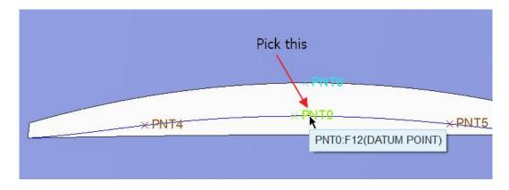
Now we will specify the tangent constraints for the ends of the curve.
