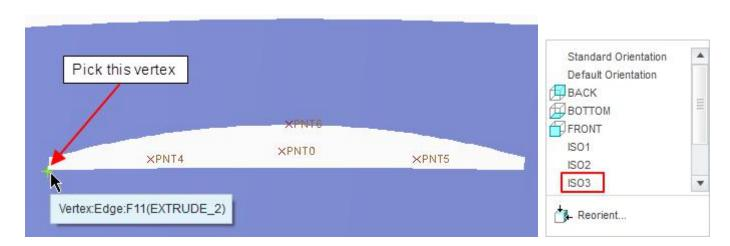
Pick the datum points one-by-one in the following order, PNT4 > PNT0 > PNT5, as shown in figure below.
