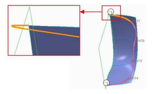
It is due to the wrong direction of normal constraint. So pick Flip to reverse the direction.
