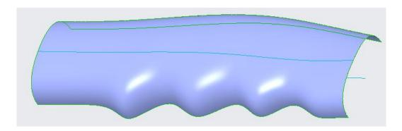
Notice that cross-section remains aligned to the chains all along the sweep feature.
