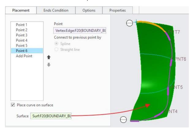
'Place curve on surface' option is used to create a spline curve that passes through the selected points and lies on a specific surface patch.
