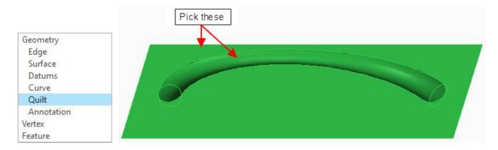
Pick Merge on the Model tab to invoke Merge tool.
