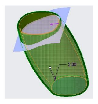
Pick icon to complete the feature. (Leave the offset type to Standard, which is default)
