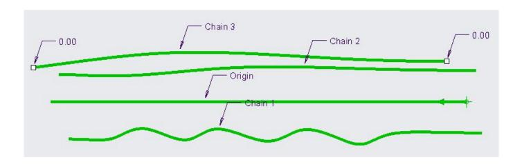
The order, in which chains are selected have no effect on the sweep geometry. Only the desired Origin Trajectory should be selected first.
