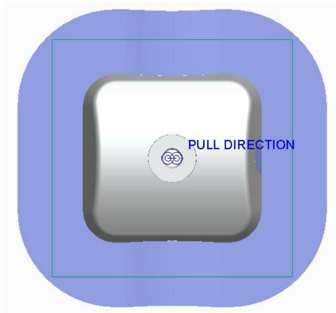
Notice that now parting surface completely intersects the workpiece.
