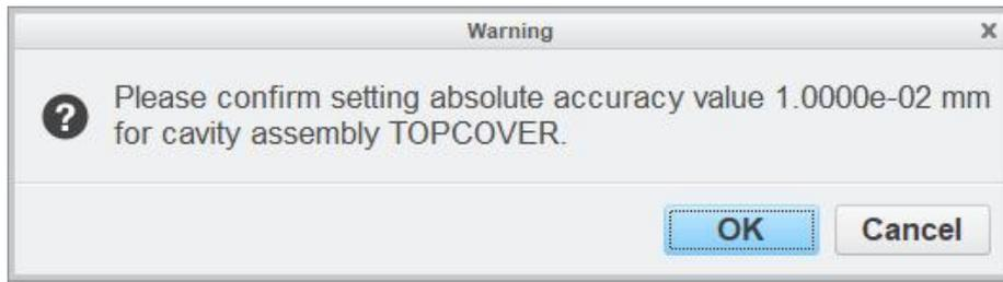
This is to change the absolute accuracy of the manufacturing model equal to that of reference model.
