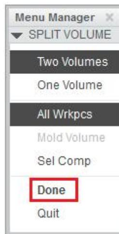
System will ask to select the parting surface for splitting the workpiece, so select the previously defined surface **PS\_FLAT** as shown below.
