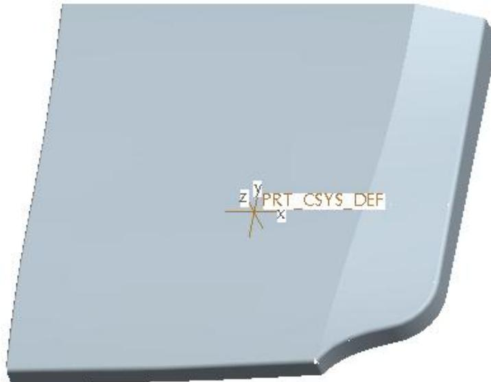
This part will be used as the design part for the manufacturing model. Notice that it has predefined coordinate system which will be used to assemble to the manufacturing assembly.
