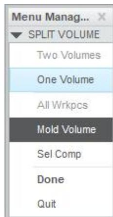
One volume split classifies the geometry to the one side of the parting surface and creates a new volume for that. The remaining geometry still belongs to the original volume that is being split.
