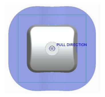
Notice that now parting surface completely intersects the workpiece.
