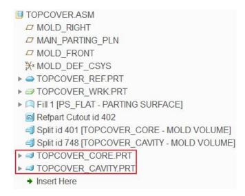
An extracted component retains associativity with the parent volume; if the volume is modified, the component is updated when the mold model is regenerated.
