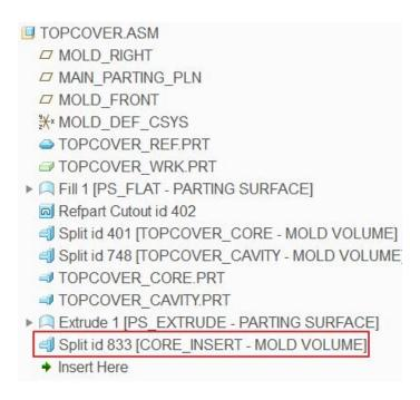
Pick Mold Display icon on the View tab and blank all the Volumes and Parting Surfaces and unblank the TOPCOVER\_CORE.PRT component.
