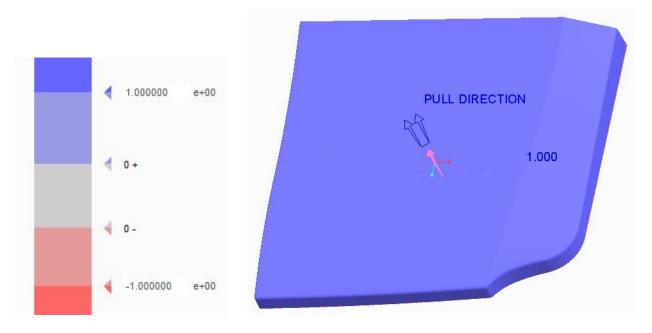
Notice that all the surfaces have more than 10 draft according to legend. The designer should decide, based upon the material to be molded and surface finish of the product, whether this draft is sufficient or not.
