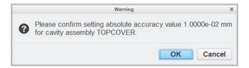
This is to change the absolute accuracy of the manufacturing model equal to that of reference model.
