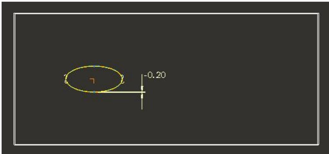
The purpose to this offset is to have clearance between the parts.
