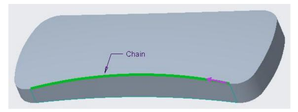
Hold down the Shift key and place the mouse pointer over any edge belonging to top surface and Right-Click to query.
