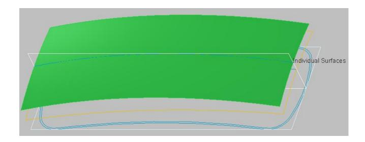
Pick in the Chain collector to activate it and select the following highlighted curve.
