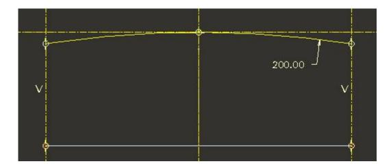
We have aligned the end points of the arc to the centerlines just to make sure that the surface generated will intersect with other features that lie within the part boundaries.
