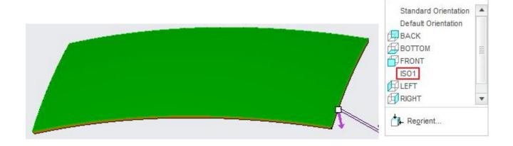
Direction of arrow should be as shown in the above figure to make sure that material is added to the desired side of surface.
