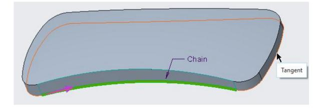
Pick in the Pull Direction collector and select the **TOP** Datum plane as reference.
