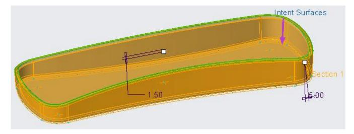
Make sure that Offset Direction arrow points in the direction shown. It will make sure that material is removed from the part.
