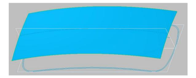
Normal To Projection option makes sure that the surface does not overlap or intersects itself and hence there is no manufacturing problem for the final components using this surface as reference.
