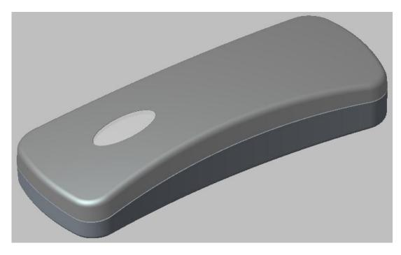
Now if you modify any dimension in the skeleton and regenerate the assembly. You will see that all the parts referencing that geometry update accordingly after regeneration.
