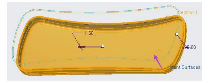
Make sure that Offset Direction arrow points in the direction shown. It will make sure that material is added to the part.
