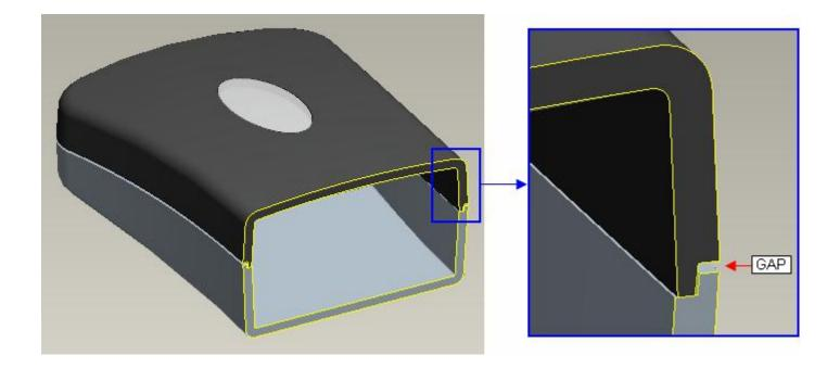
You should notice the gap between Top and Bottom halves. The purpose of this gap is to disguise any mismatch due to manufacturing tolerances between these parts.
