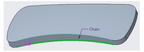
Hold down the Shift key and place the mouse pointer over any edge forming the bottom surface and Right-Click to query.
