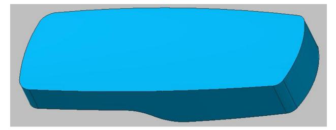
Now we will apply the split draft to the side surfaces so that TOP and BOTTOM parts are manufacturable using injection molding process. The side surfaces will be split about the split surface (the surface at which both components join). To achieve this, we need to create a datum curve to be used as neutral curve.
