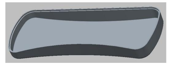
Now we will create an offset feature that will create a gap between top and bottom halves to disguise any mismatch between both parts.
