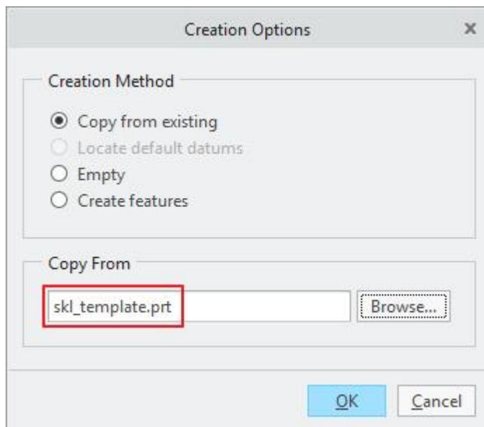
SKL\_TEMPLATE.PRT is the template file that contains the default datum features, layers and accuracy settings.
