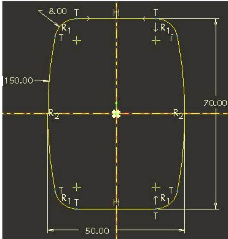
Make sure that centerlines are aligned to the datum planes and Scale should be set to 1 as shown below.
