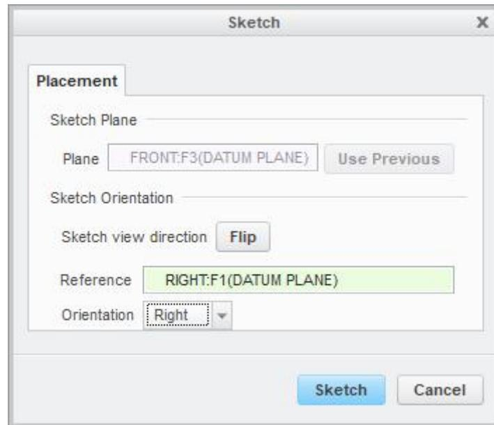
Select the following references for dimensioning and constraining the section geometry.
