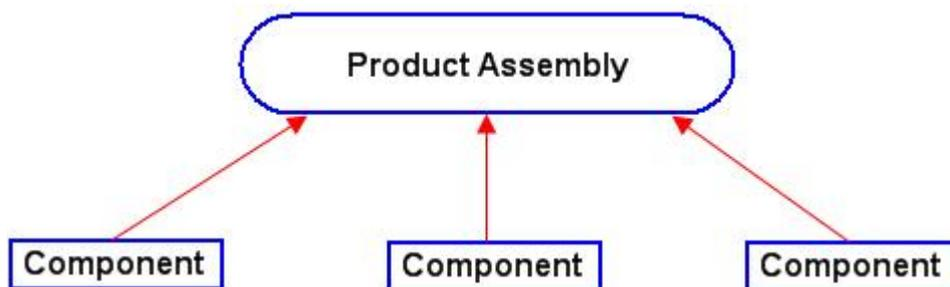
It is a manual approach to ensure that components fit properly and meet the design criteria. First the individual parts are designed in great detail. The parts are then assembled together to form assemblies of a product. Components are independent of each other. So that if one component is modified, the related components have to be changed manually.
