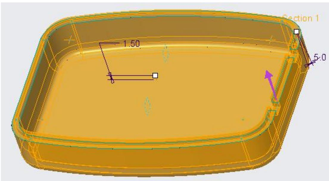
Make sure that Offset Direction arrow points in the direction shown. It will make sure that material is added to the part.
