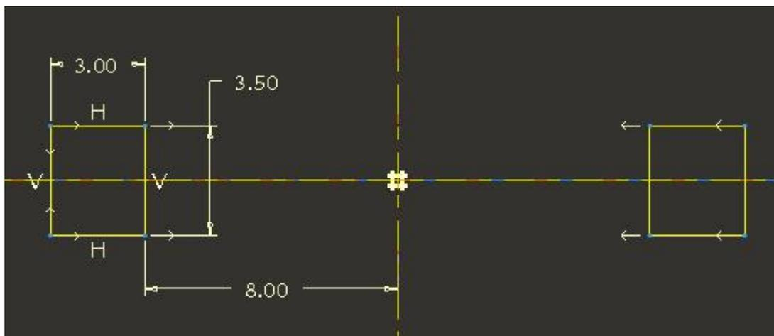
Make sure that centerlines are aligned to the datum planes.
