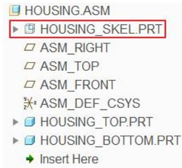
A skeleton model can be created at any time in the design process. The system always inserts the newly created skeleton model before all other components and assembly features.
