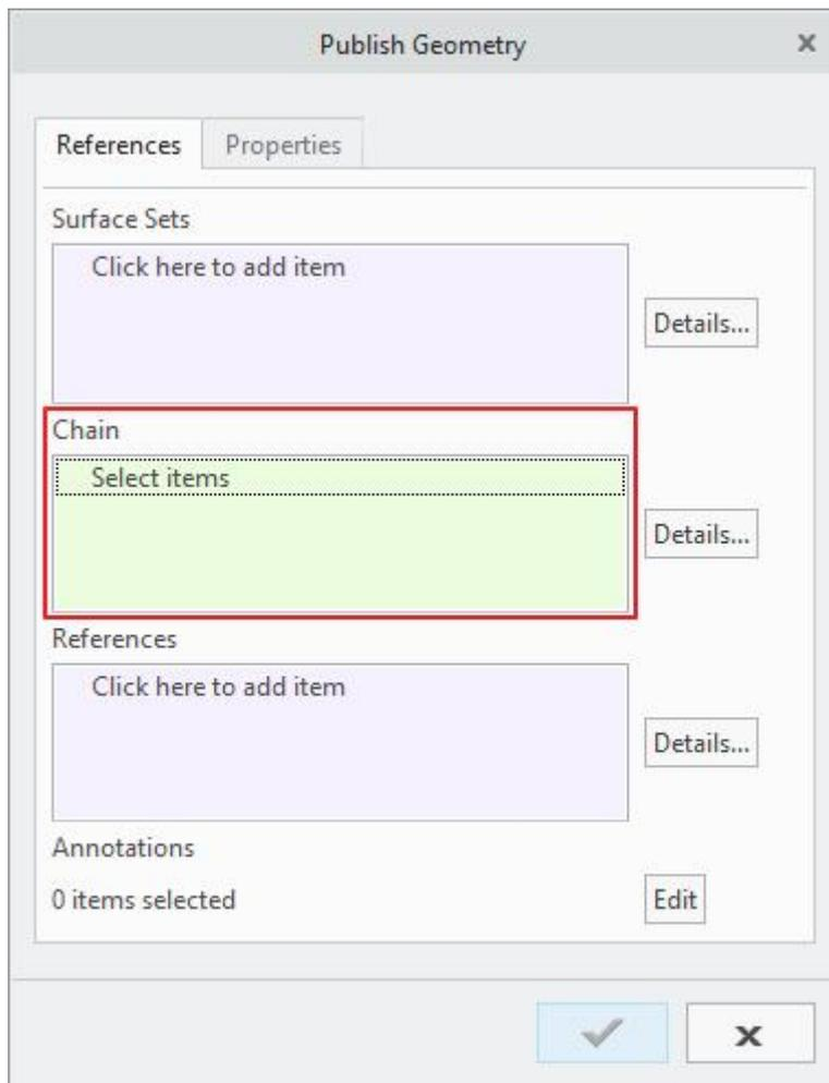
Hold down the Ctrl key and pick all the datum curves in the skeleton model as shown below
