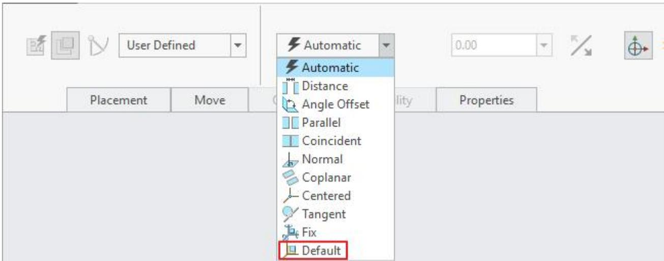
The Default constraint aligns the default system-created coordinate system of the component to the default system-created coordinate system of the assembly.
