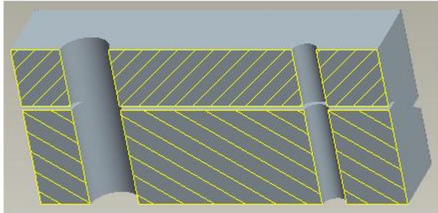
You should notice that geometry in both parts update according to the changes made in the skeleton.
