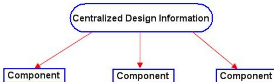
Top-down design (TDD) approach allows to control the relations of components with each other so that if one component changes the related components change automatically. If implemented properly you can have full control of the assembly at a central location.
