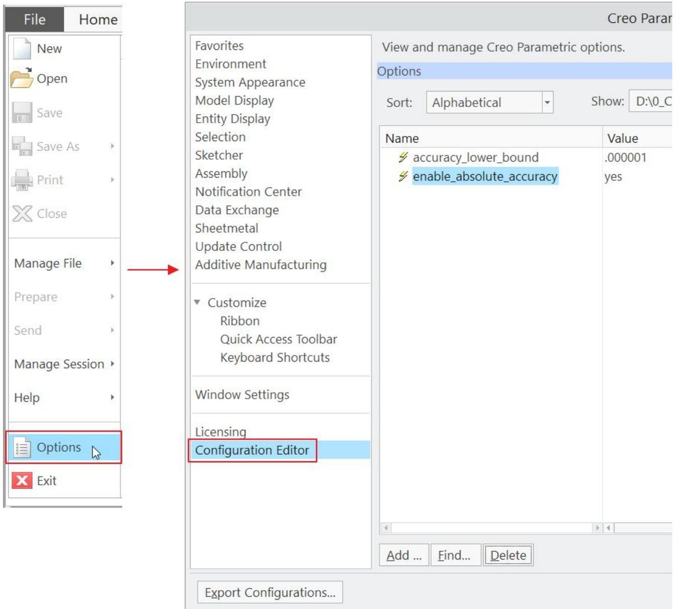
accuracy\_lower\_bound value is used to override the default lower accuracy limit of 0.0001
