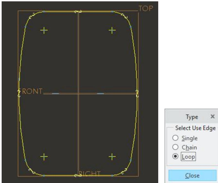
After completing the sketch specify the blind depth of **12** in the direction as shown below. (Note that extrusion direction is towards brown side of the datum plane/positive direction of y-axis. Set the view to **ISO2** to avoid any ambiguity.)
