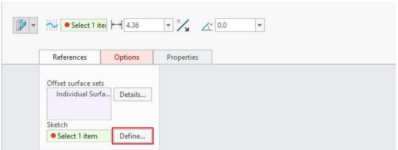
Select the sketching references as shown below. Also flip the direction of sketch plane for clear view.
