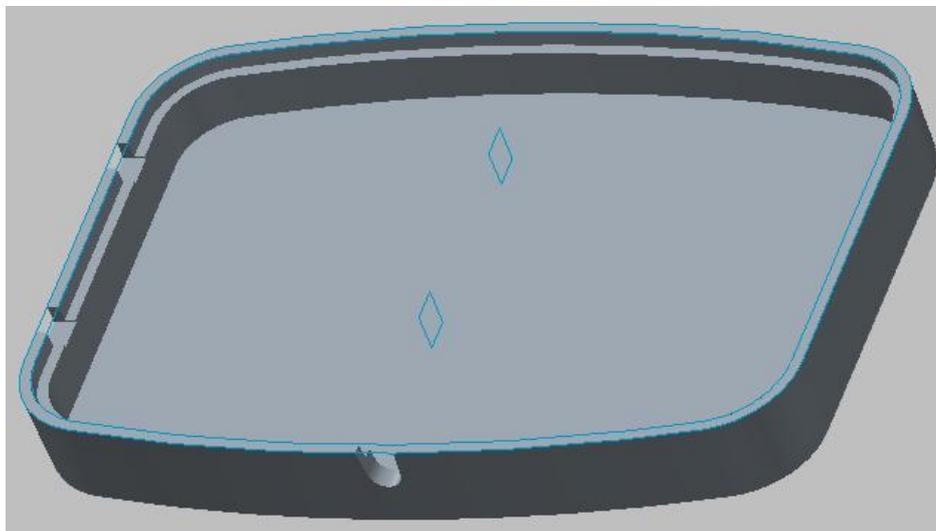
Now we will create an offset feature that will create a gap between top and bottom halves to disguise any mismatch between both parts.
