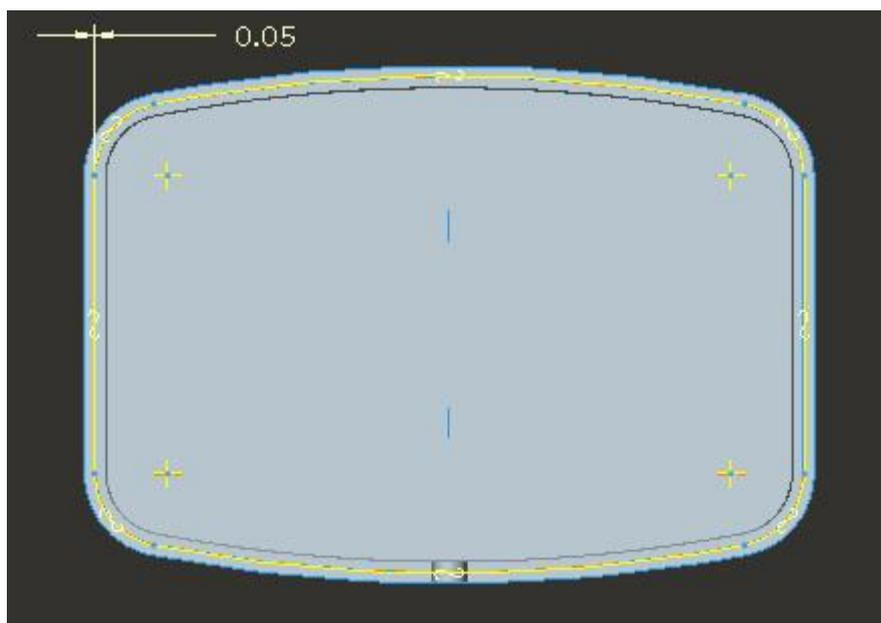
The purpose to this offset is to have some clearance between lip geometry of both parts.
