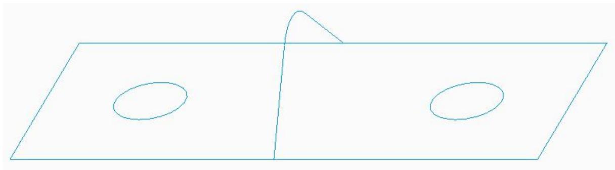
These datum curves will be used to drive the geometry in individual components according to design intent. Both components will reference these curves therefore the relationship or common attributes between the components will always be maintained.
