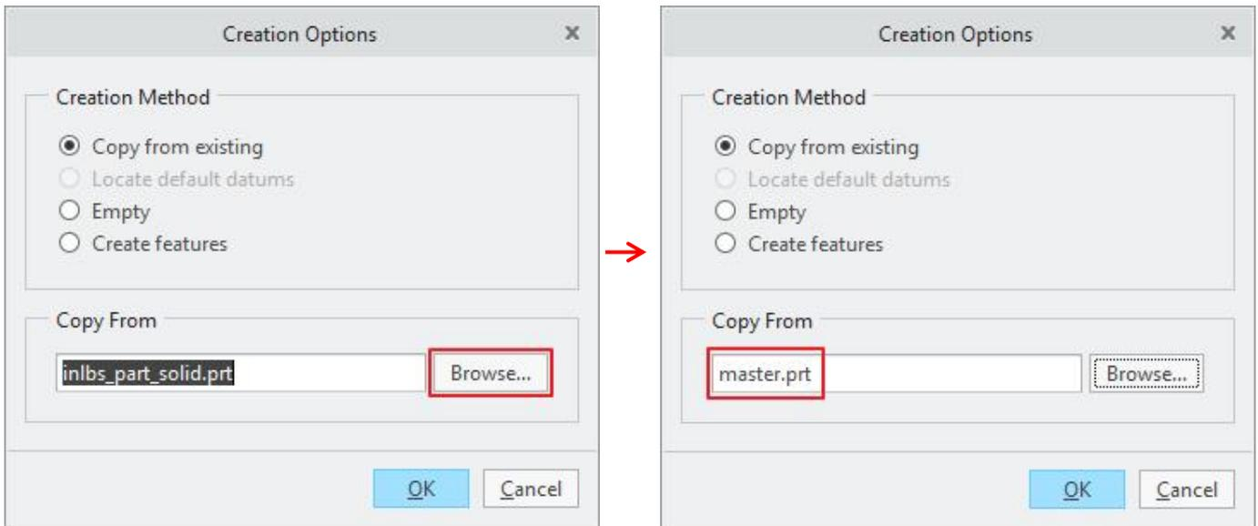
MASTER.PRT is a regular Creo part that contains the geometry that we want to use in our skeleton model. Although you can create that geometry directly in the skeleton part but for convenience it has already been created in this part. Skeleton part is just copying the geometry from this existing part.
