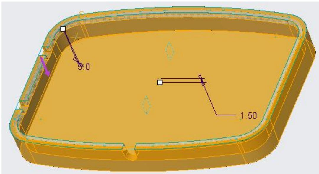
Make sure that Offset Direction arrow points in the direction shown. It will make sure that material is removed from the part.
