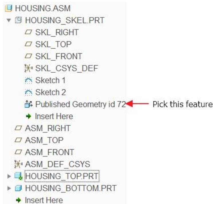
When you create a Copy Geometry feature, you can reference either individual references like curve, surface and datum features or a Publish Geometry feature.
