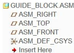
We will assemble two empty components and then create the geometry that will be driven by a skeleton. After completing the components, the assembly will appear as shown below.
