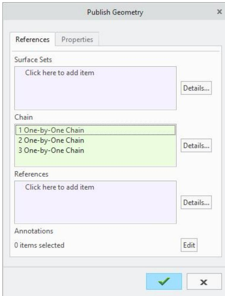
Publish geometry feature allows to mark the references, in a source part, that can be referenced by a copy geometry feature altogether. So it is a consolidation of multiple local references that can be copied to other models.
