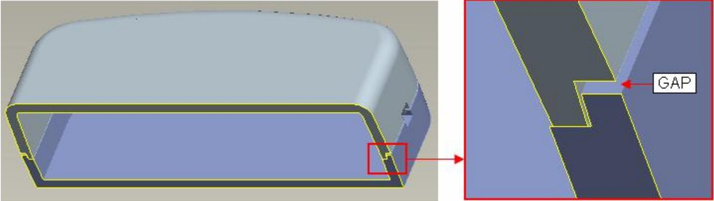
You should notice the gap between Top and Bottom halves. The purpose of this gap is to disguise any mismatch between these parts.
