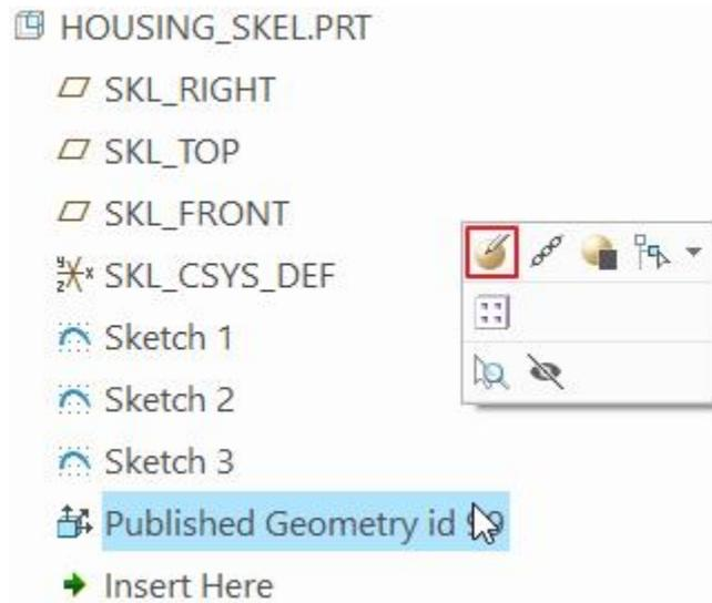
Activate the Chains collector and pick the curve formed by SKETCH\_3 feature while holding down the Ctrl key.
