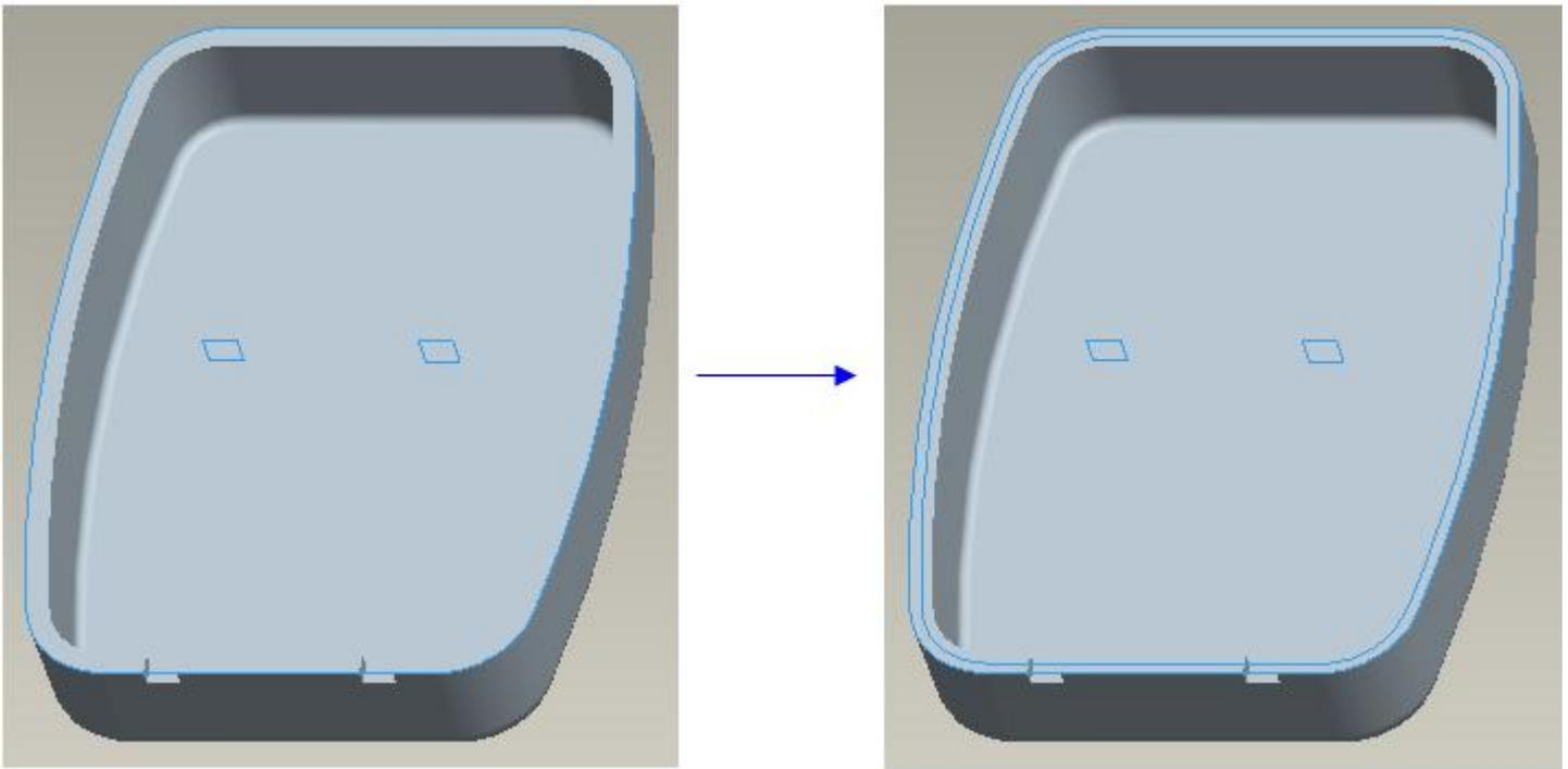
It is because the copy geometry feature in this part is referring the publish geometry feature in the skeleton model. Therefore the geometry added or removed in publish geometry feature will be reflected here.
