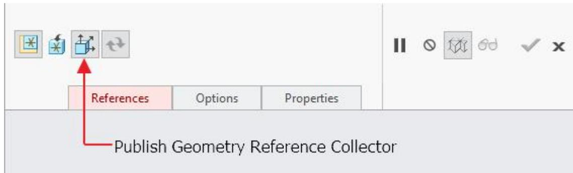
Notice that Publish Geometry reference collector is active by default. So select the publish geometry feature in the skeleton part by picking it in the model tree as shown below.
