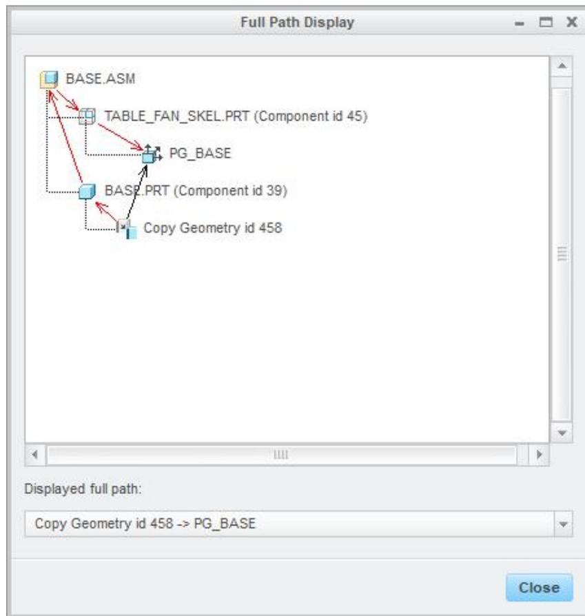
It can be seen that the copy geometry is referencing published geometry feature in the skeleton model in the context of the assembly. So the system will need the skeleton and BASE assembly in session to update and regenerate this part when the skeleton is modified.
