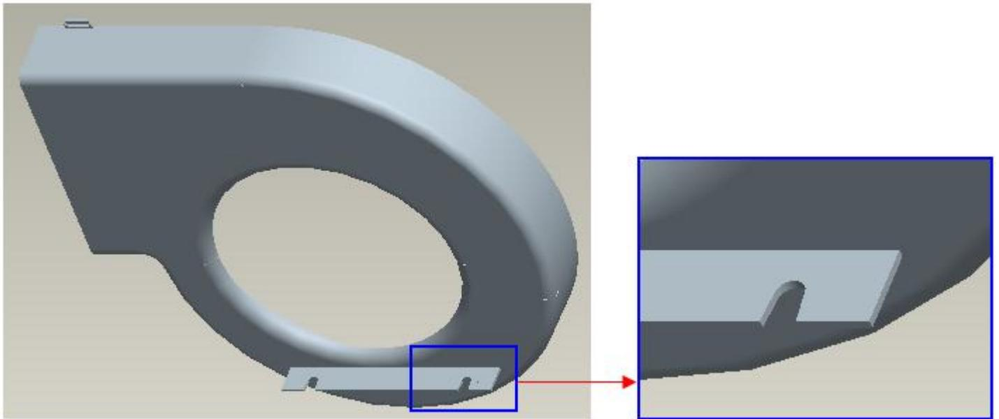
If you open the MOTOR\_BASE.PRT in a new window and regenerate the part, you can see the new sketched circles appearing there. You can create the bosses using those circles as references on your own. After creating the bosses the part will appear as shown below.
