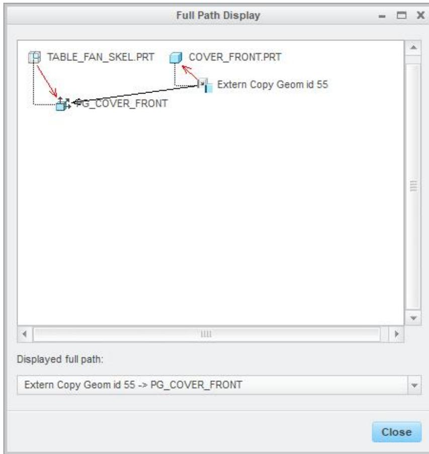
It can be seen that the external copy geometry feature in COVER\_FRONT is referencing the Publish Geometry feature in the TABLE\_FAN\_SKEL part without assembly context. So the system will only need the skeleton in session to update and regenerate this part when the skeleton is modified. Therefore we can use this method without pulling all parts and assemblies into session. So a part using external copy geometry will require very few resources of the computer to update and regenerate it.
