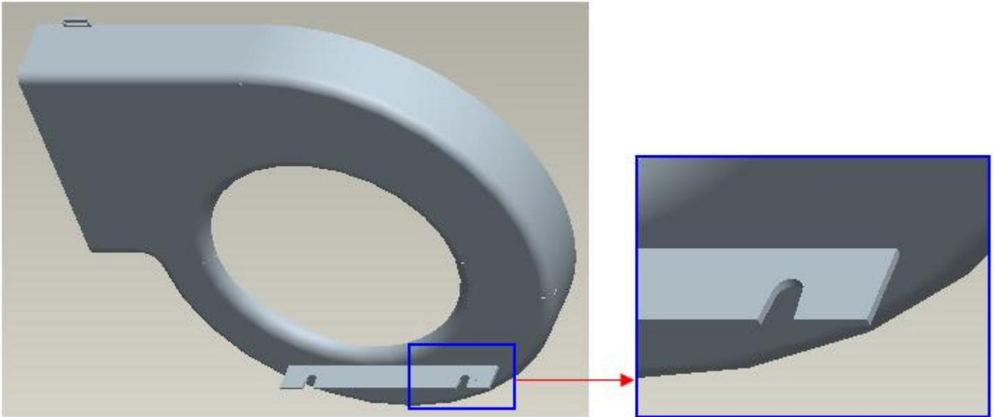
The cut features in HOUSING\_LEFT and bosses in MOTOR\_BASE should be aligned. So we need to create the geometry in a skeleton that both parts can reference.
