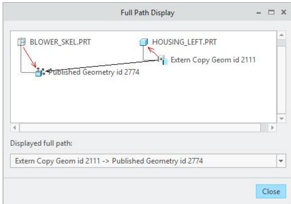
It can be seen that the parent of the external copy geometry feature in HOUSING\_LEFT.PRT is the Publish Geometry feature in the BLOWER\_SKEL.PRT without any dependency on the assembly.
