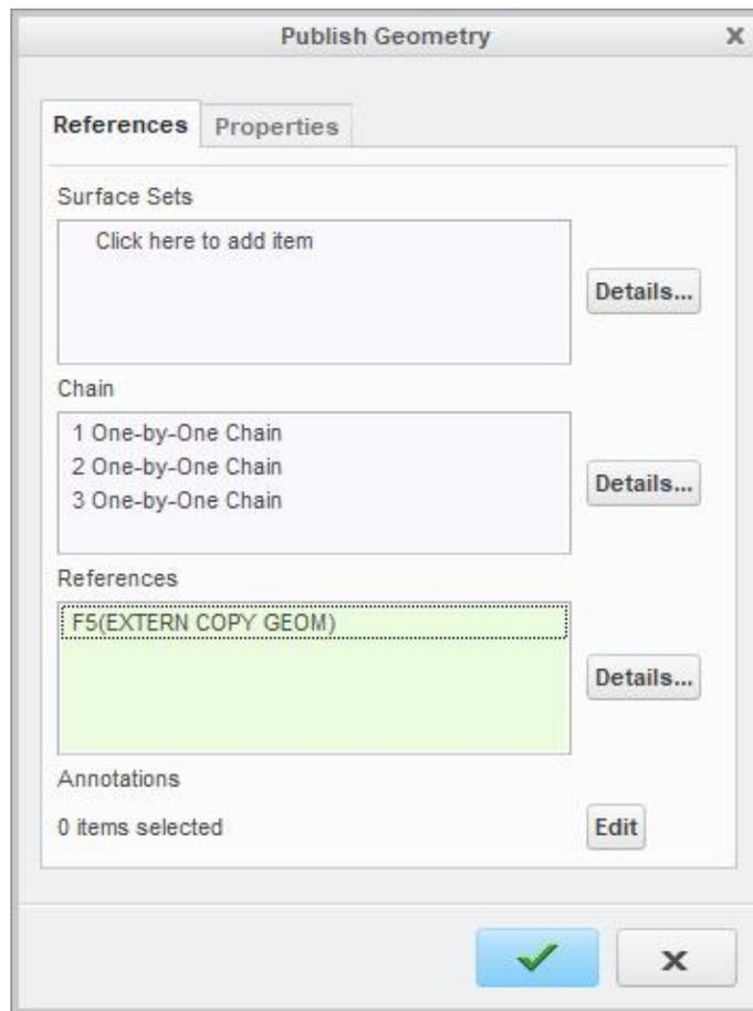
If complete copy geometry feature is not required, we can copy the required geometry belonging to a copy geometry feature by using the Surface and Chain collectors.
