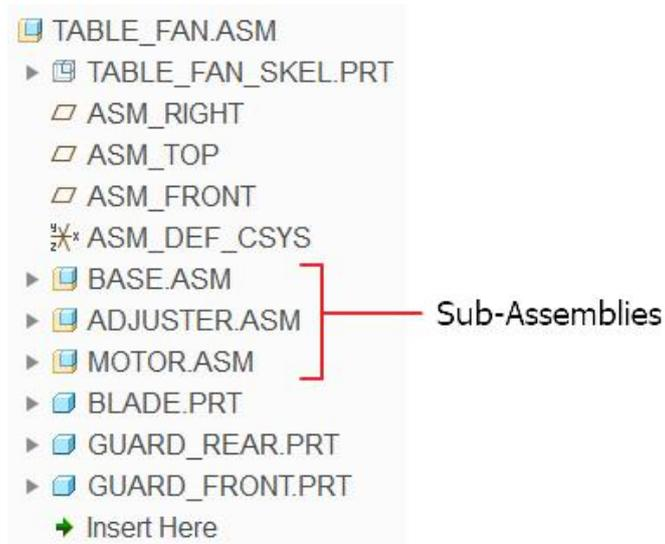
In the following paragraphs, we will see how to communicate references from the skeleton to the parts, at different level in the assembly.
