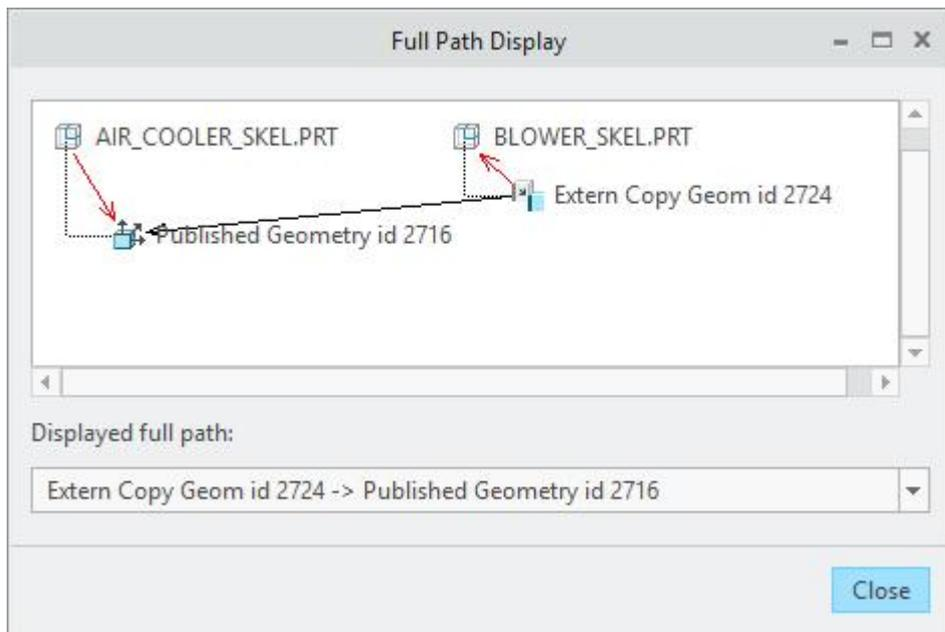
Notice that parent of the external copy geometry feature in BLOWER\_SKEL is the publish geometry feature in AIR\_COOLER\_SKEL without any dependency on the assembly. So system will only need AIR\_COOLER\_SKEL in session to update and regenerate BLOWER\_SKEL when any change is made in AIR\_COOLER\_SKEL.
