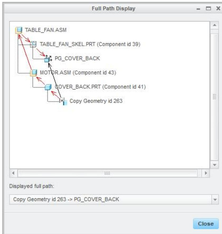
It can be seen that the parent of the copy geometry feature in COVER\_BACK is the Publish Geometry feature in the TABLE\_FAN\_SKEL part in the context of the TABLE\_FAN.ASM. So the system will need the skeleton and TABLE\_FAN assembly in session to update and regenerate this part when the skeleton is modified. Therefore this method should never be used to copy references to a part as it requires the complete main assembly in session to propagate a change from skeleton.
