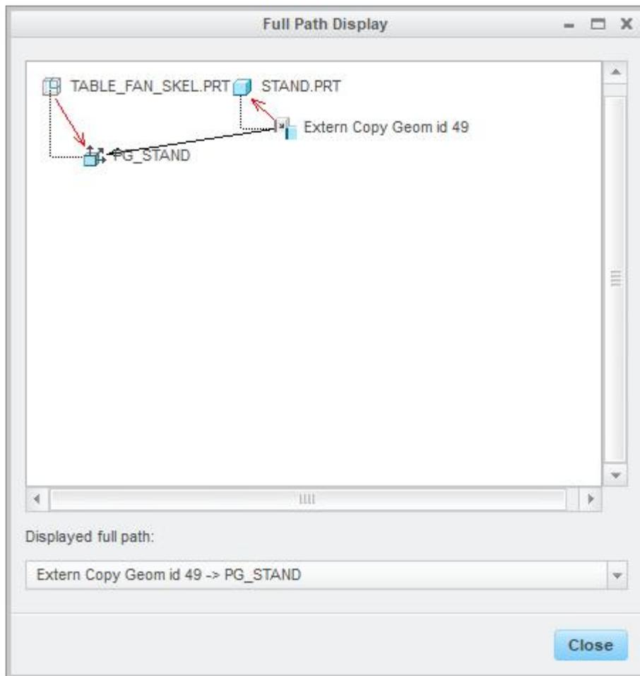
It can be seen that STAND.PRT has no dependency on the assembly. So the system will only need the skeleton in session to update and regenerate this part when the skeleton is modified.
