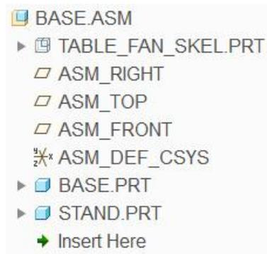
Now we will create the Copy Geometry feature in the BASE.PRT that is located in BASE.ASM
