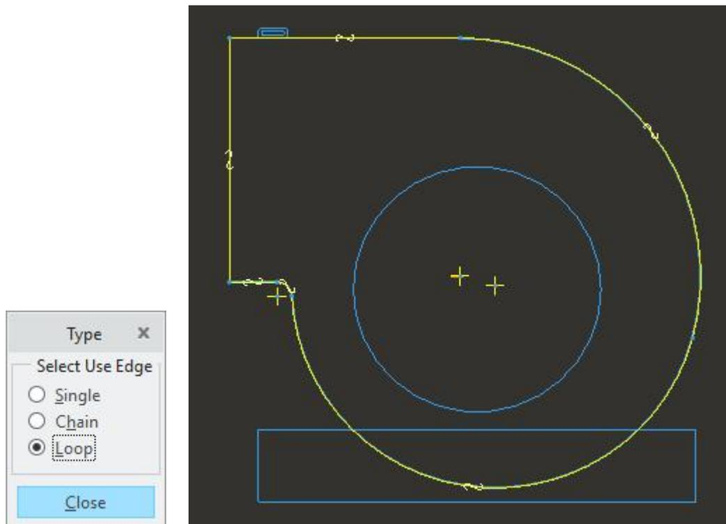
After completing the sketch, change the depth option to **To Selected** (
